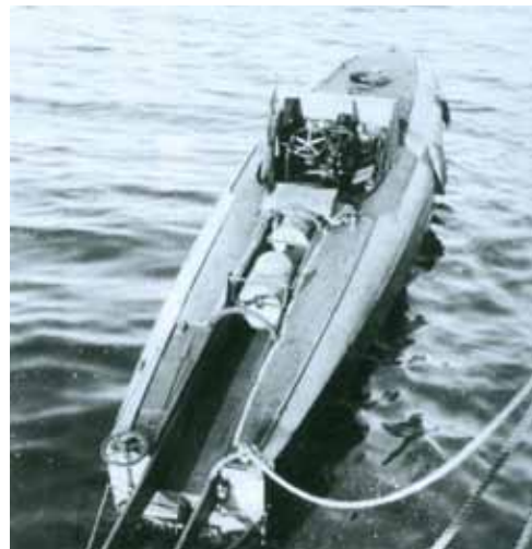
40 Ft. CMB4 Cockpit & Torpedo Slot
